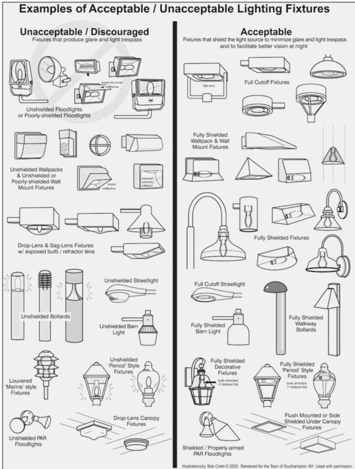
Figure 04-2: Full Cutoff Light Fixture Examples 179
